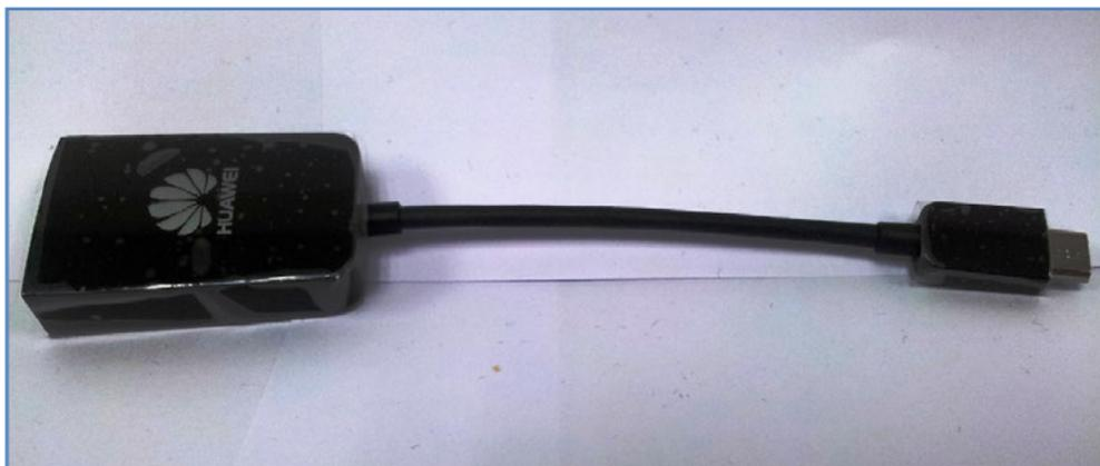
When connected to the portable AF10, E5756/E5776 act as a charger that supply power to devices such as a mobile phone, MP3, MP4, or Bluetooth headset
